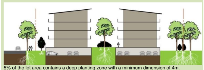
5% of the lot area contains a deep planting zone with a minimum dimension of 4m.
