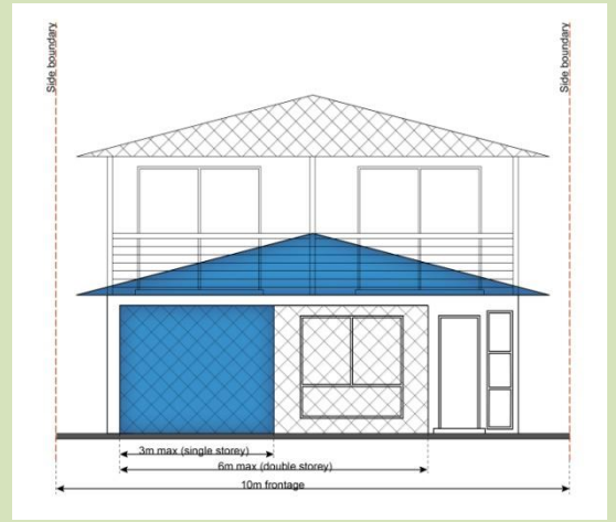
Example: Dwelling house – lot frontage less than 12.5m non-laneway frontage. Single storey is 3m if no porch/portico or the like, double storey is 6m.
