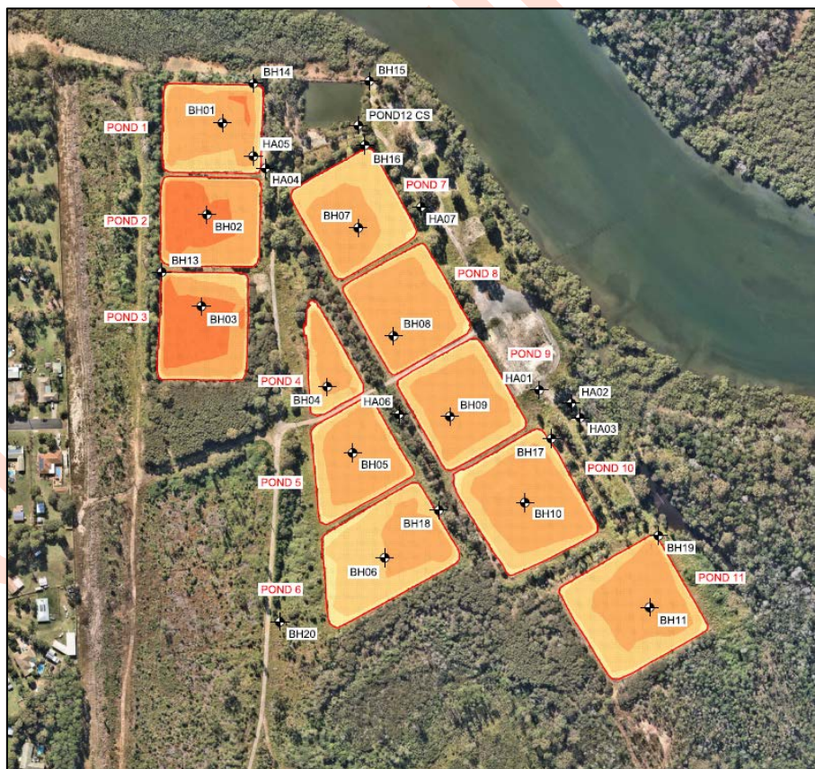
Figure 2 Pacific Harbour Maintenance Dredging project - Ningi dredged material placement site - 'pond' layout
